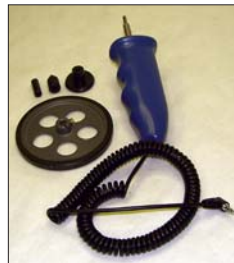
Remote Infrared Sensor (IRS-P) Gap 0.50 inches
